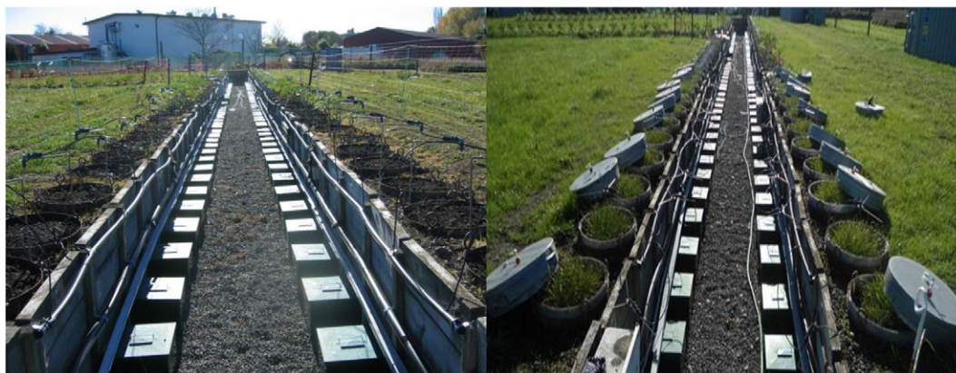
Fig. 1. Left—Installation of lysimeters; Right: Gas chambers just before the gas collection.
