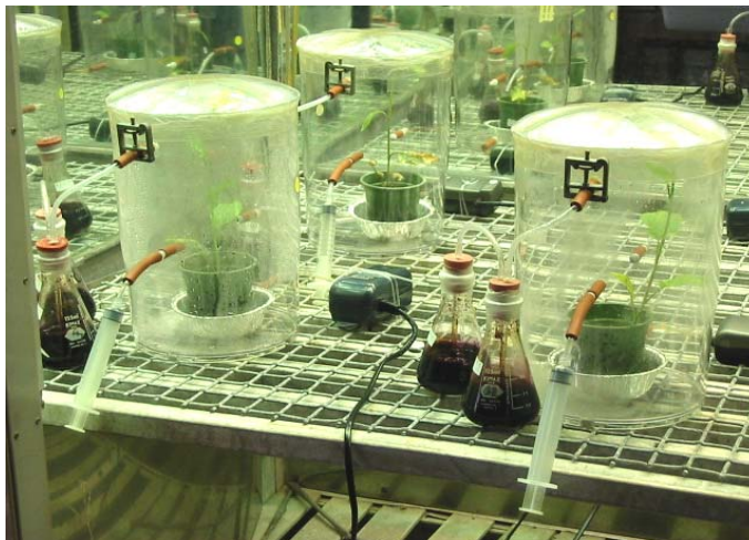
Figure 13. Gastight volatilisation chambers used for trapping volatile Hg released from the plant-substrate system. B. juncea plants grown on Tui, modified Gold Mountain (GM) and Serra Pelada (SP) substrates were treated either with (\text{NH}_4)_2\text{S}_2\text{O}_3 or \text{NH}_4\text{SCN} and immediately enclosed within the chambers.
