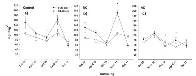
**Fig. 3.** Evolution in time of water soluble carbon (WSC) in the three studied soils and at two different depths (0–20 cm and 20–40 cm). Mean values  $\pm$  standard error (n = 3). Significant differences between depths for each soil and time are marked with an asterisk.
