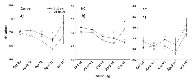
**Fig. 1.** Evolution in time of soil pH (graphs a, b and c) at the three studied soils and at two different depths (0–20 cm and 20–40 cm). Mean values  $\pm$  standard error (n = 3). Significant differences between depths for each soil and time are marked with an asterisk.
