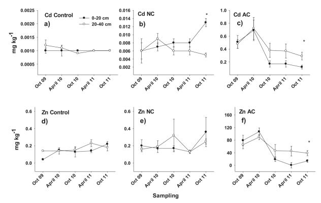
**Fig. 2.** Evolution in time of available Cd and Zn extracted with 0.01M CaCl<sub>2</sub> (graphs a, b and c) at the three studied soils and at two different depths (0–20 cm and 20–40 cm). Mean values  $\pm$  standard error (n = 3). Significant differences between depths for each soil and time are marked with an asterisk.
