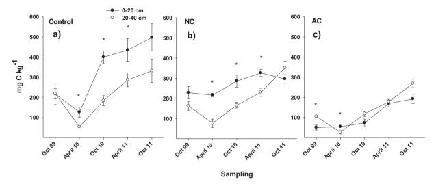
**Fig. 4.** Evolution in time of Microbial Biomass Carbon (MBC) in the three studied soils and at two different depths (0–20 cm and 20–40 cm). Mean values  $\pm$  standard error (n = 3). Significant differences between depths for each soil and time are marked with an asterisk.
