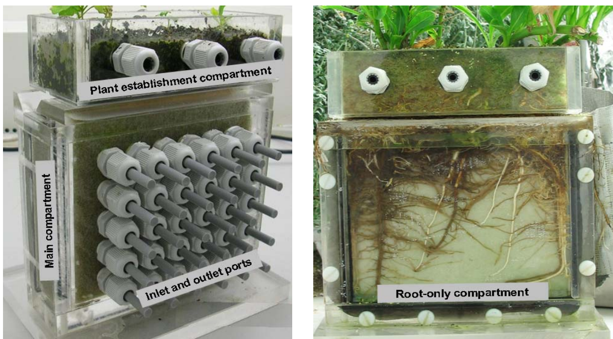
Figure 3.1: The rhizobox set up with a view of the outlet and inlet ports (left) and the root-only compartment (right)
