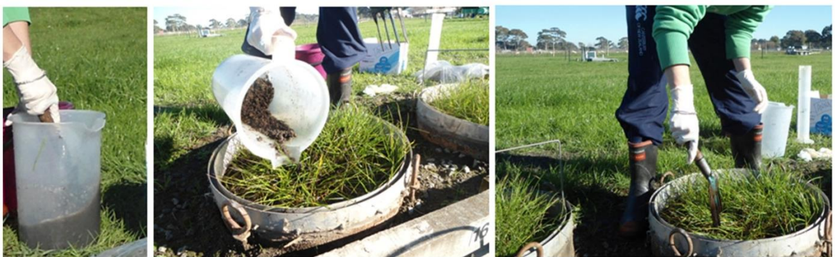
Figure 3-2. Homogenising of biosolids and lignite prior to application (Left), Treatment application (middle) and evenly distributing treatment across the lysimeter surface (right).
