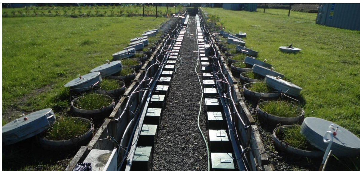
Figure 3-1. Lysimeter trench (lysimeters 1-18) prior to N 2 O gas collection.
