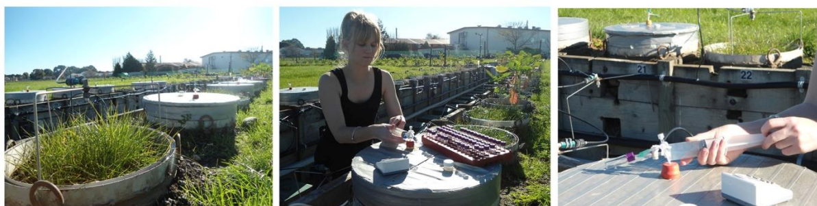
Figure 3-3. Lysimeters with and without gas collection chamber (left). Collection of gas samples (middle) and gas sampling syringe and needle setup (right).
