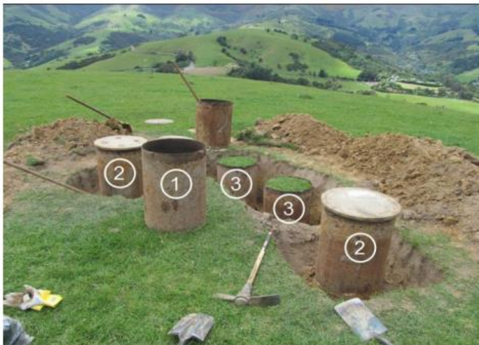
Figure 22. Photo showing the stages of lysimeter sample collection. (1) the lysimeter is placed on the sample soil. (2) the lysimeter is dug into the ground. (3) the lysimeter is ready to be removed from the sample site.
