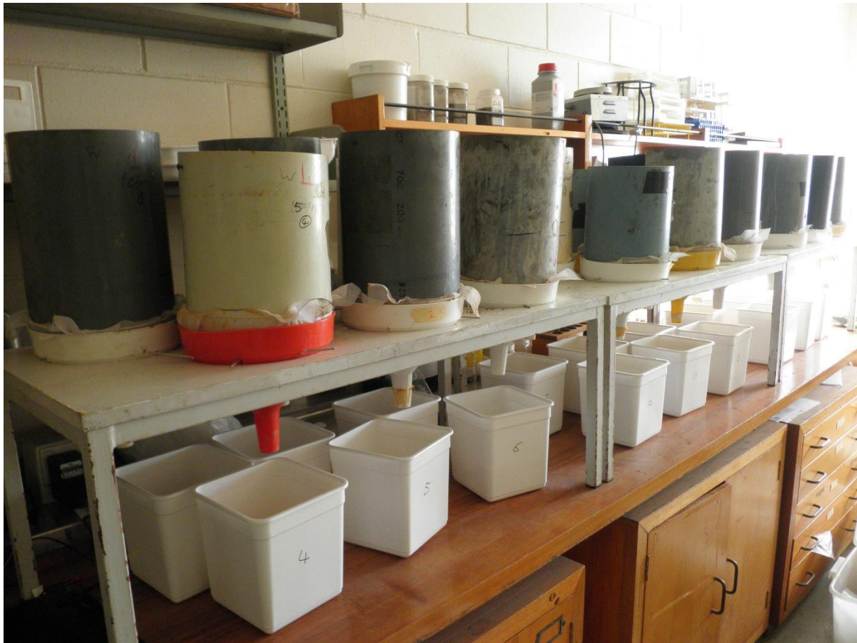
Figure 19. Photo of soil column set up in lab. Soil columns are set up above drainage collection buckets.
