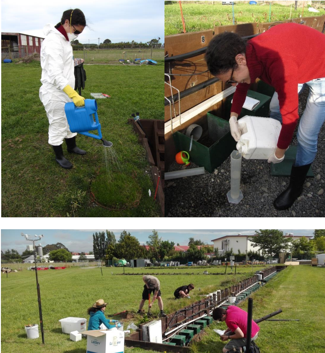
Figure 23. Opposite: The installed lysimeters showing the six Pawson silt loam soil cores (front-left) and the 12 Barry's soil cores (rear-right). Top left: Effluent application. Top right: Drainage collection. Bottom: Destructive sampling of the lysimeters at the conclusion of the experiment. 16 th of November, 2016.
