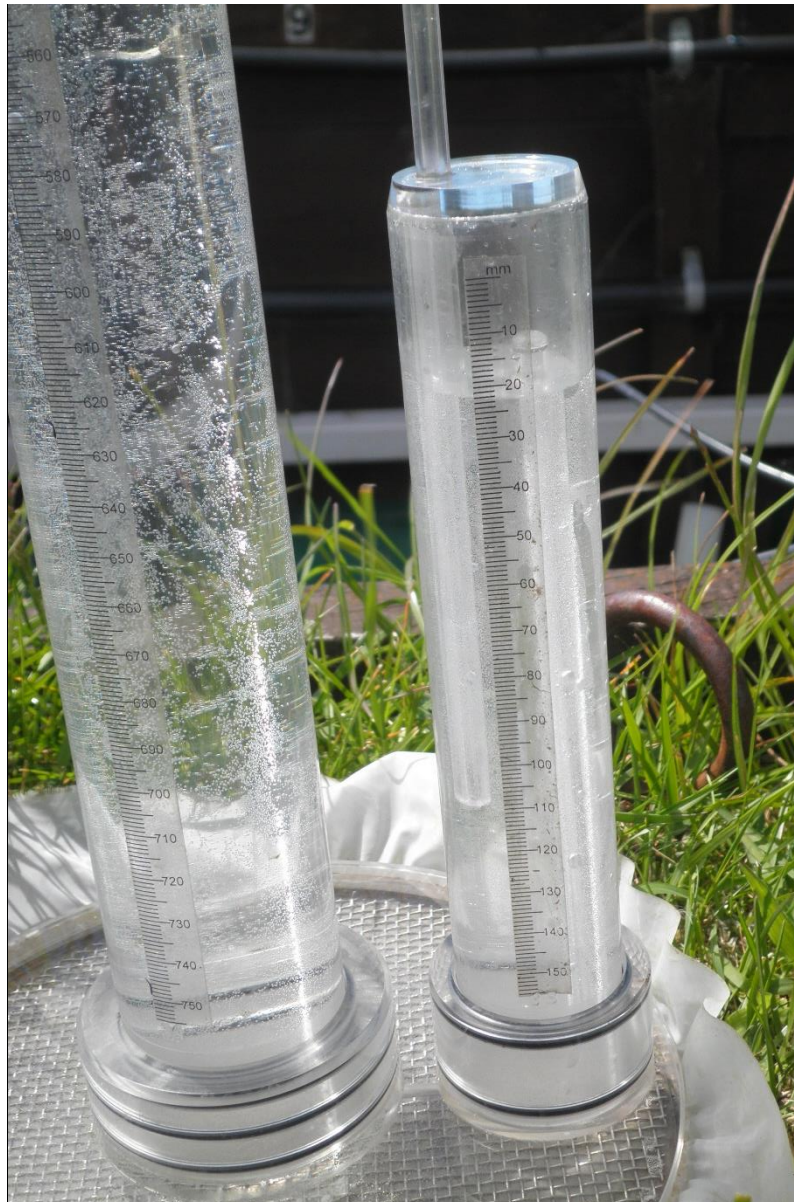
Figure 24. Opposite: Pasture cleared from the lysimeter surface in preparation for the disk permeameter, Opposite bottom: Infiltration rate data collection using a disk permeameter, Above: Water reserve and bubble tower set to -10.0 cm pressure.
