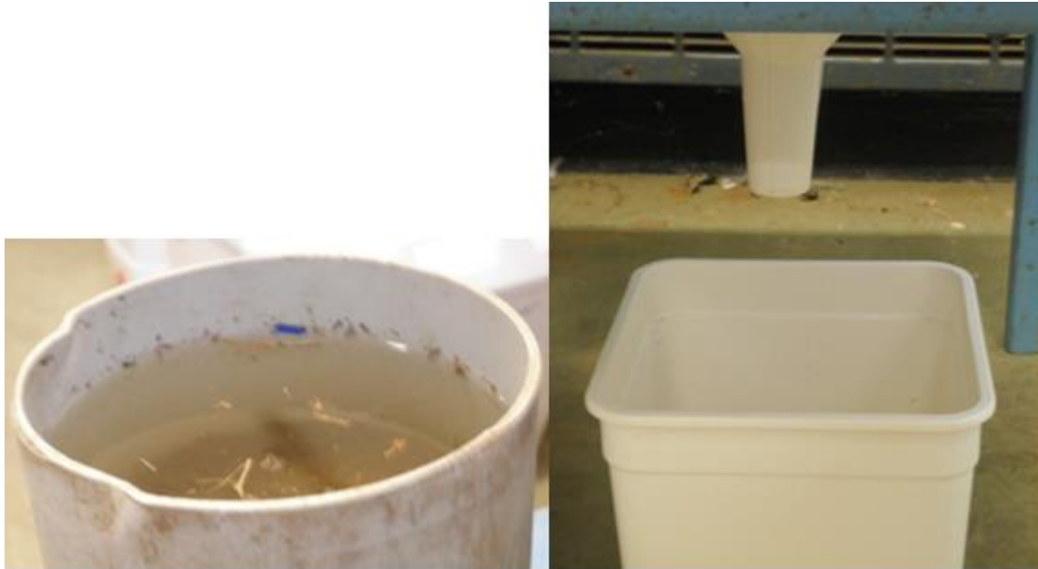
Figure 21. Left: Soil column under a constant head of 50 mm of water, Right: Steady state of drainage being collected from the soil column.
