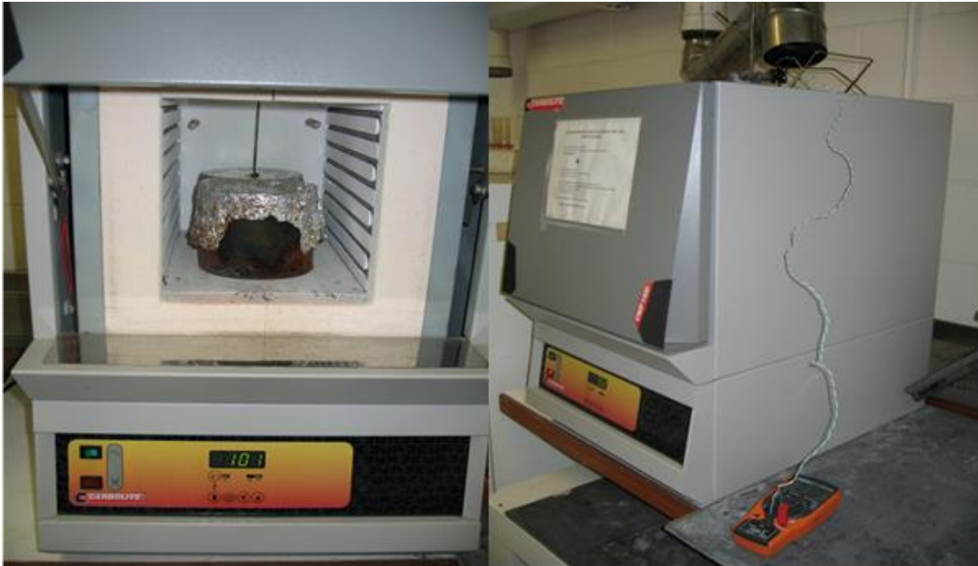
Figure 4-8. Furnace equipped with a thermocouple and exhaust ventilator.
