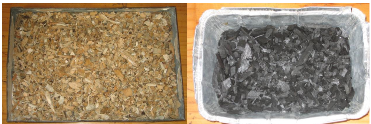
Figure 4-7. Pine wood-waste (left) and biochar pyrolyzed at 400°C with steam activation (right). NB- There was no distinguishable visual difference between steam activation and non-activated.
