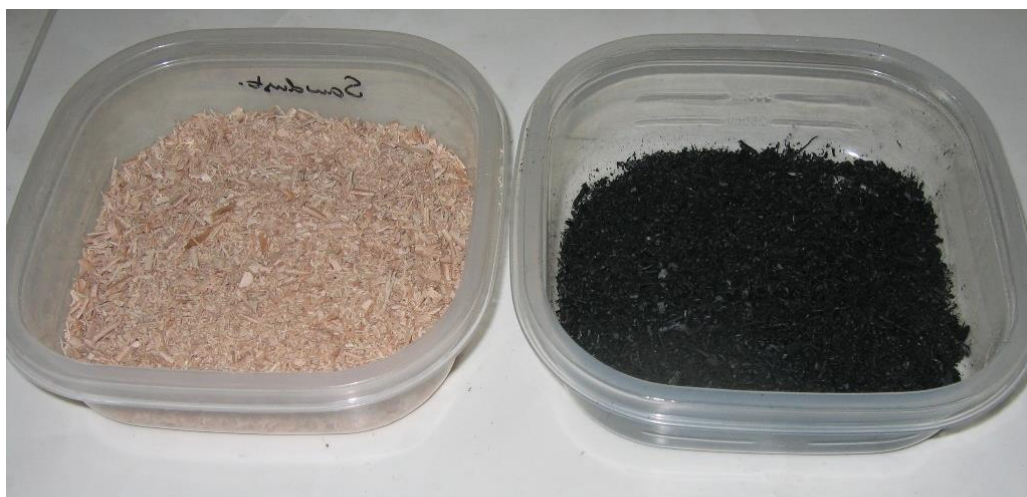
Figure 4-11. Kanuka sawdust and biochar manufactured at 350°C (3 hr).
