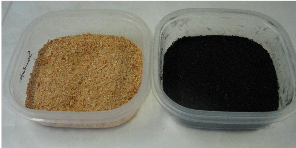
Figure 4-9. Pine sawdust (left) and biochar manufactured at 350°C (3hr) (right).
