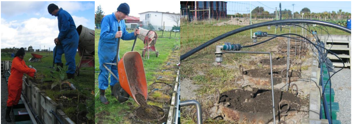
Figure B. 4. Left- Right: Top 10 cm lysimeter soil was removed; mixed with treatment and placed back in the lysimeter with the help of my supervisor Brett Robinson; each lysimeter was equipped with the irrigation system.
