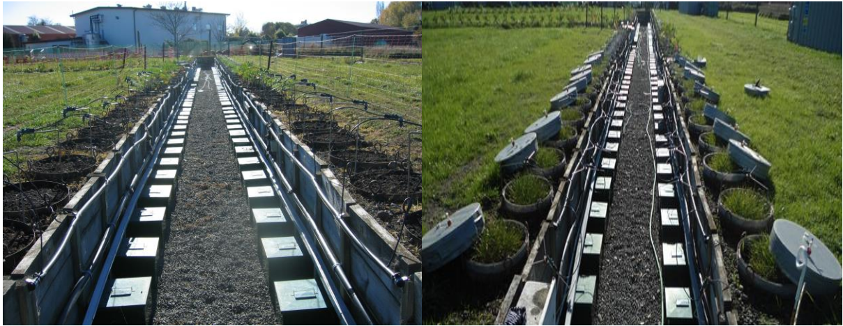
Figure 6-1. Left : Installation of lysimeters; Right : Gas chambers just before the gas collection.
