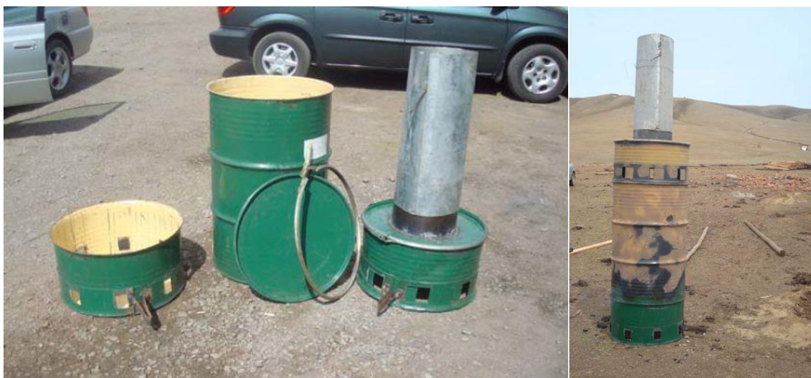
Figure 8-6. Left : Oil barrel pyrolyzer components, Right : fully assembled pyrolyzer (Munkhbat et al., 2012).
