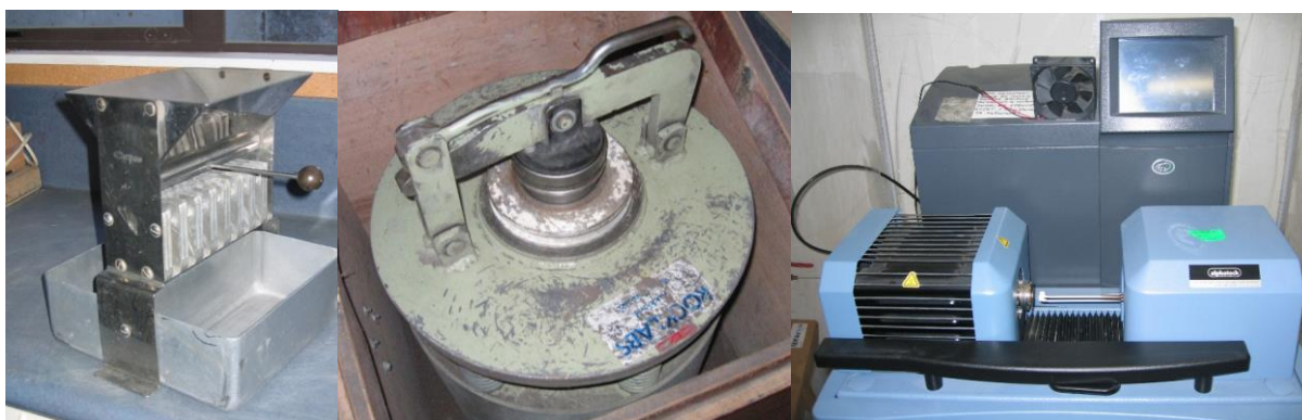
Figure 4-12. Left to Right : Sample homogenizer; sample grinder; TG analyzer.
