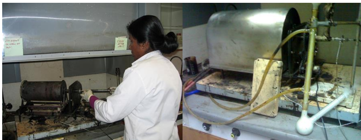
Figure 4-5. Left -Setting-up the pyrolyzer; Right - During the pyrolysis, waste crude tar was collected in a two-necked round bottom flask.
