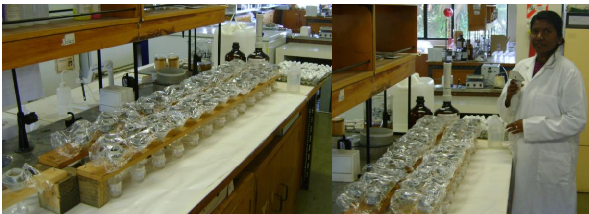
Figure A. 2. Column leaching experiment in the laboratory.
