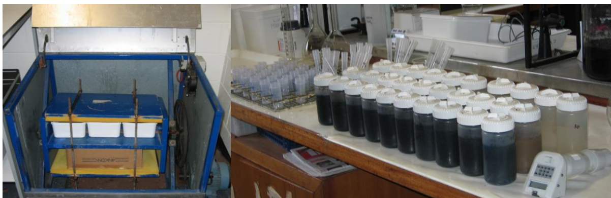
Figure A. 1. Left - End-over-end shaker; Right - Sorption samples ready for a timely sub-sampling
