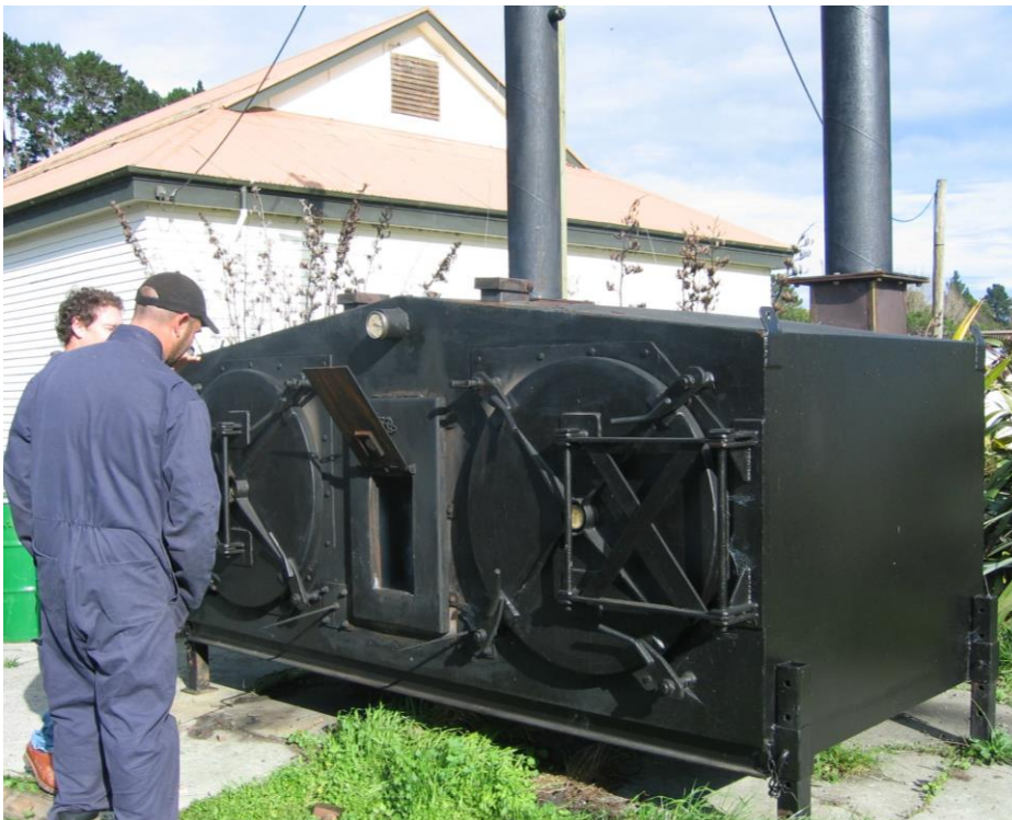
Figure 8-5. The pyrolyzer at Palmerston North belongs to the New Zealand Biochar Research Centre (When I visited this site in 2011 it was being installed, photo by Dharini on the 10/04/2011).
