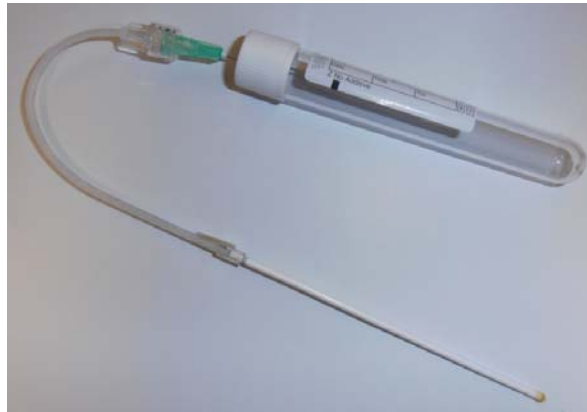
Plate 9- Photograph of fully assembled rhizon sampler coupled with a syringe and vacuum tube.
