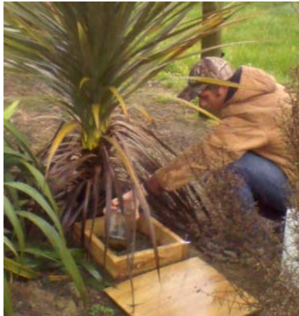
Plate 11. Application of effluent slurry to sampling sites. (Photograph by N. Dickinson, personal communication, 2011)
