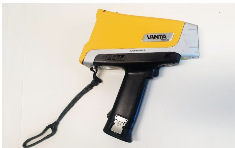
Figure 3.8. M series Vanta XRF analyzer that was used for in-situ field testing of soils in the RZ.
