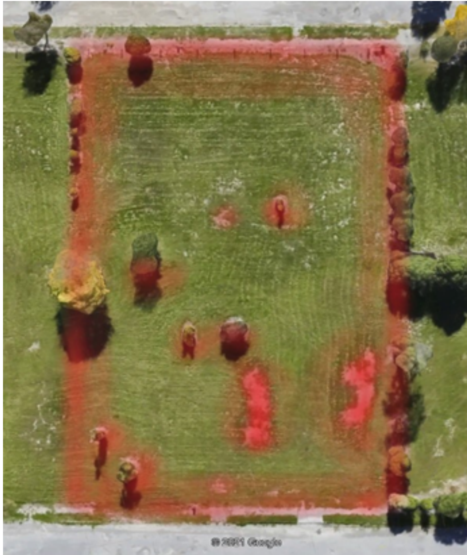
Figure 3.10. Aerial map of a Red Zone property in Avondale that shows the areas of interest when conducting targeted sampling. Note. The red highlighting represents the areas of high priority when measuring HM concentrations in RZ soils. The highest concentration of HMs is expected to occur in the areas highlighted in red. Adapted from a base image from Google Earth Pro using Paint 3D.
