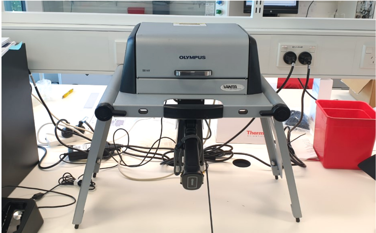
Figure 3.9. Photograph of the Vanta workstation that was used for calibration (XRF analyzer is connected underneath).
