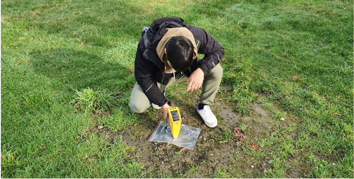
Figure 3.12. Photograph of the XRF handheld analyzer in action, at site 1 (Oxford Terrace, Christchurch Central City).
