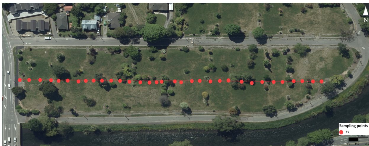
Figure 3.7. Layout of a transect sampling campaign. Note. The red dots represent the transect sample locations and the red line represents the ideal path to take when transect sampling. Adapted from a base map of NZ 10m Satellite Imagery (2018-2019) and Paint 3D.
