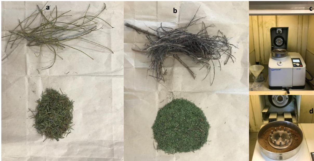
Plate 7. 4 Dried leaves of L. scoparium (a) and K. serotina (b) separated from branches and grinder Retch ZM200 for grinding the samples (c, d)
