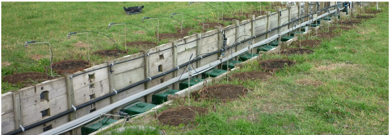
Plate 2.1: The lysimeter trench facility in the field laboratory.
