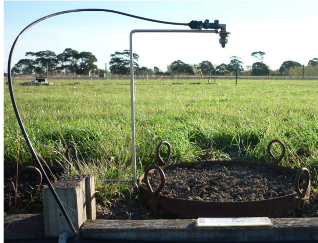
Plate 2.2: The irrigation system supplying automated water to each lysimeter.
