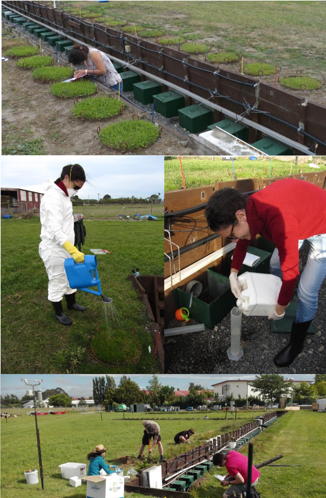
Fig. 3. Top: The installed lysimeters showing the six Pawson silt loam soil cores (front-left) and the 12 Barry's soil cores (rear-right). Centre left: Effluent application. Centre right: Drainage collection. Bottom: Destructive sampling of the lysimeters at the conclusion of the experiment. 16 th of November, 2016.
