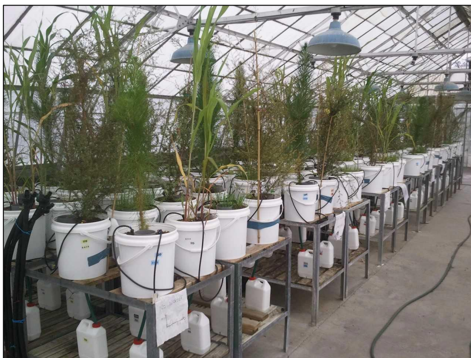
Figure 3.2 The pots (small lysimeters) arrangement and automatic irrigation system in Exp. 1.
