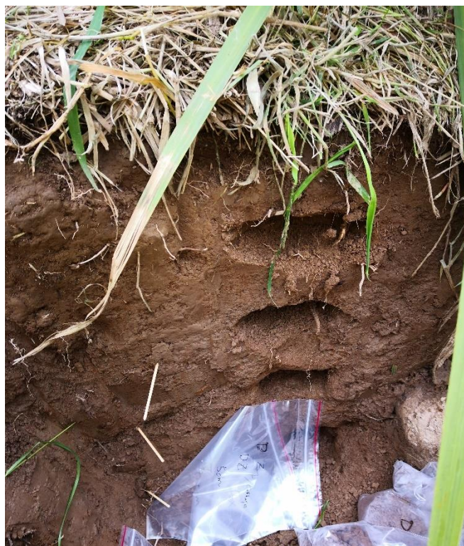
Figure 3: Sample collection from a soil pit.
